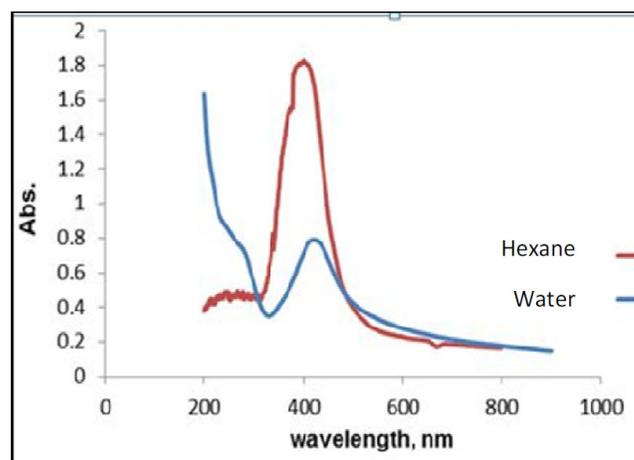
Fig. 1 : UV-Visiblespectroscopy of silver Nano particles
