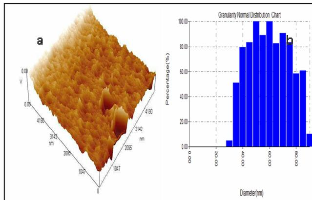
**Fig. 5 :** Three-dimensional image of silver Nano particles was synthesized by Olive oil (a) and granularity report (b).
