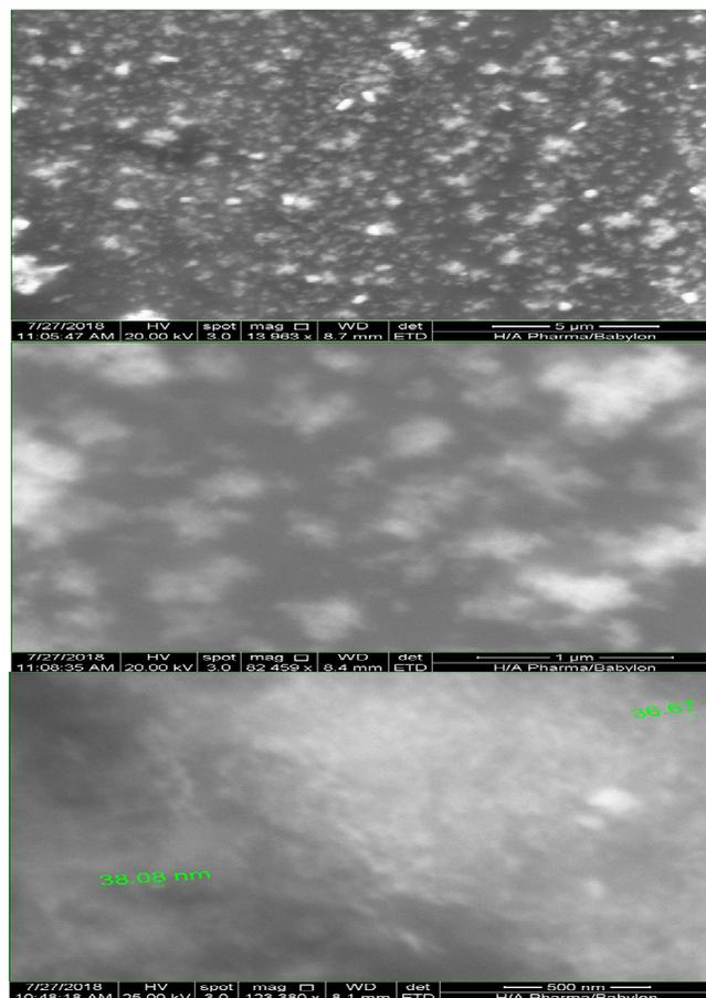
**Fig. 4 :** SEM image of synthesized AgNPS by Olive oil in three scales 5, 1 and 0.5  $\mu$ m
