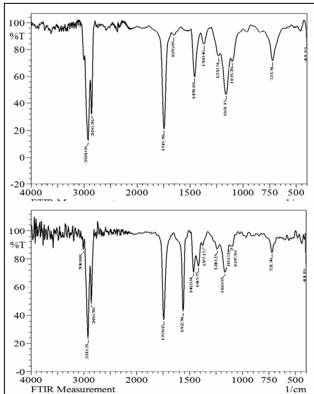
**Fig. 2:** FTIR analysis of biosynthesized silver nanoparticles by oil olive
